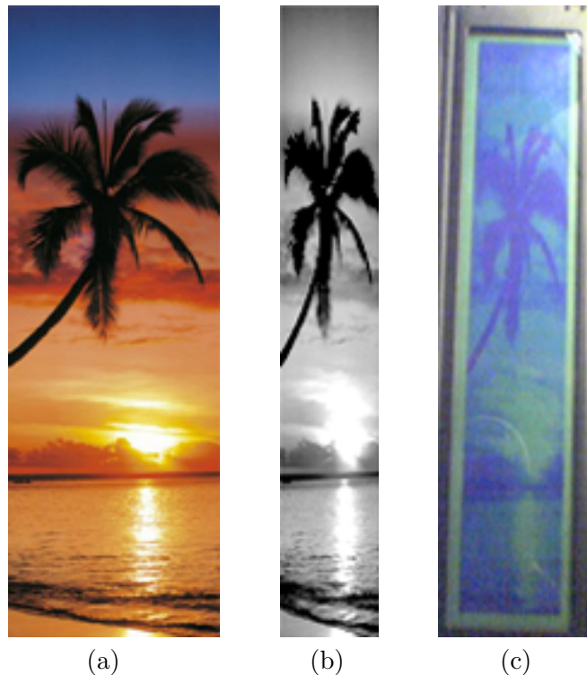
Figure 3: (a) Original image, (b) Bitmap sent to LCD (c) Simulated grayscale image displayed on LCD
